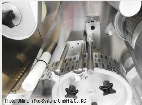
Foreign body detection in blister packs
