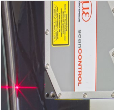
Gap measurement on car bodies
