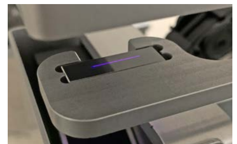
Fully automatic calibration enables reliable measurements (here: thicknessGAUGE C.LP)
